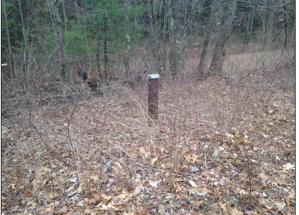
A photograph showing a single monitoring well in a field. The well is a vertical pipe with a white cap, surrounded by dry, brown leaf litter and bare ground. It is located in the foreground, with a dense forest of mostly bare trees in the background. |
