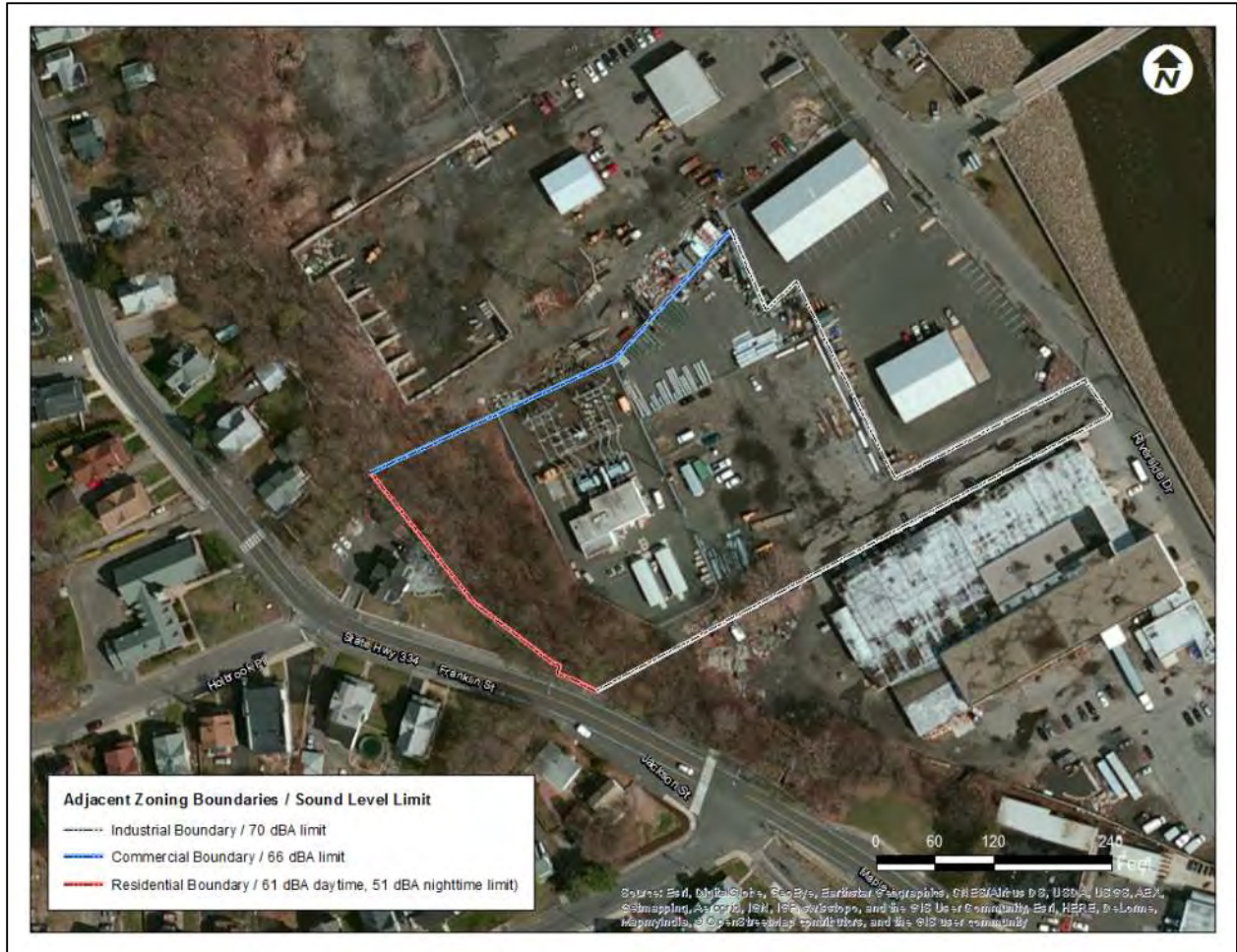
Figure 3-1 Substation sound level limits
