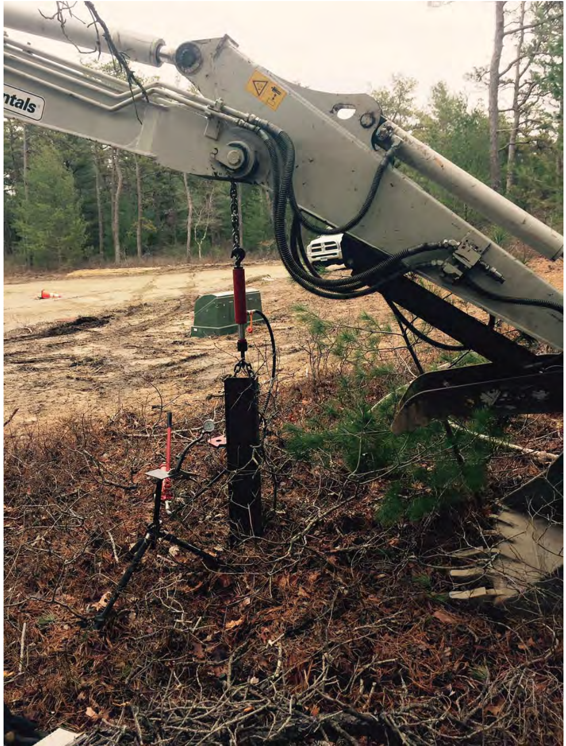
Figure 2: View of the setup used to measure axial tension.
