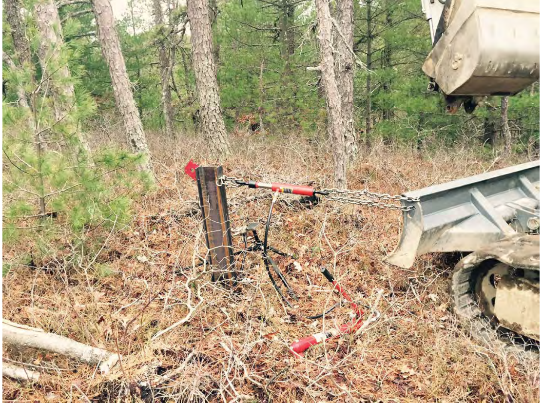
Figure 3: View of the setup used to measure shear capacity.
