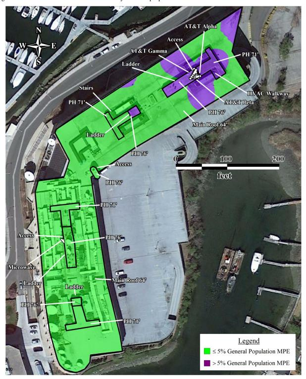
Figure 10: Predicted 5% Levels on Rooftop - AT&T Antennas Only (Full Rooftop View)
