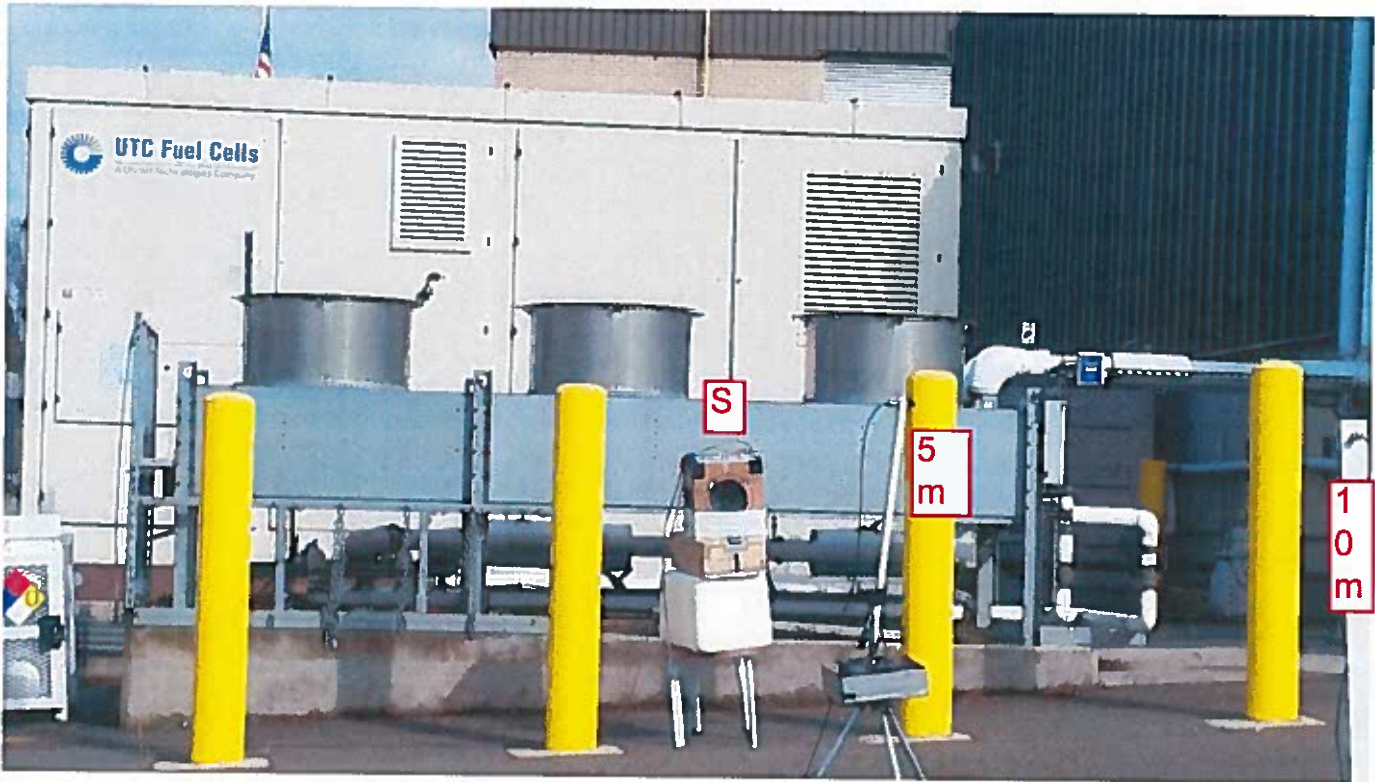
Figure 3. Speaker Source at Position S where the Fuel Cell Power Module Will Be Located
