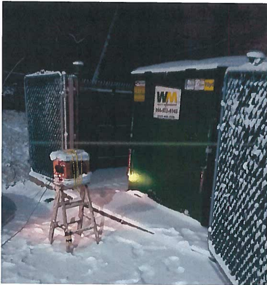
Figure 3. Speakers Used as a Simulated Airborne Noise Source at Position G
