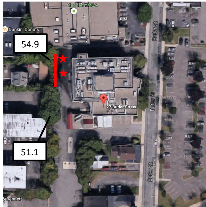
Figure 5: Satellite view of the project site identifying the location of recommended barrier wall (red line) and the location of the fuel cells. Numbers indicate the predicted sound level due to the fuel cells (in dBA).
