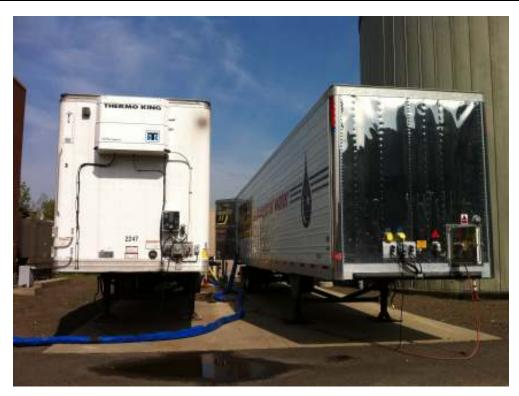
**Photograph No. 25**Demineralized water trailers and mobile treatment system.
