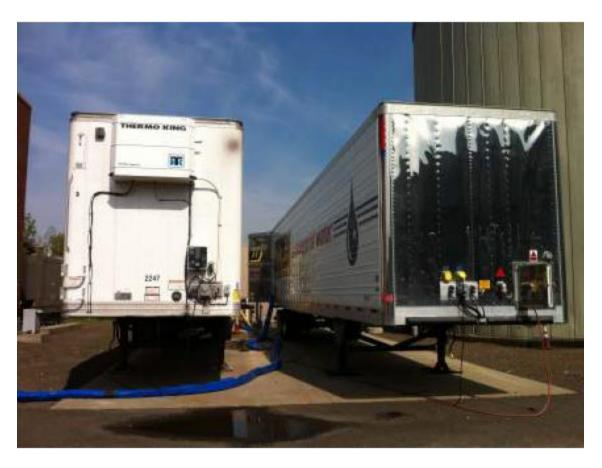
Photograph 15: Demineralized water trailers and mobile treatment system
