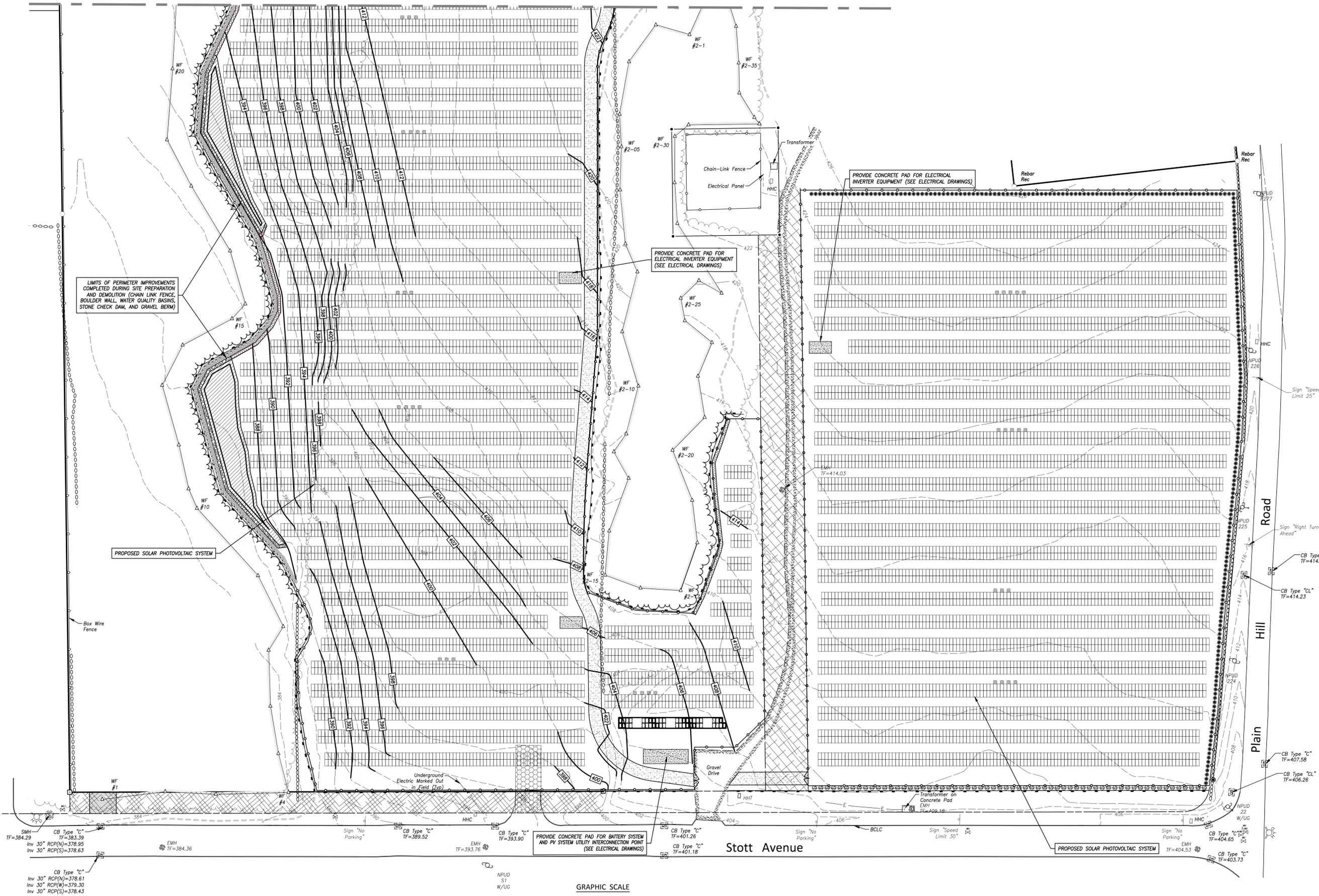
LIMITS OF PERIMETER IMPROVEMENTS COMPLETED DURING SITE PREPARATION AND DEMOLITION (CHAIN LINK FENCE, BOULDER WALL, WATER QUALITY BASINS, STONE CHECK DAM, AND GRAVEL BERM)
