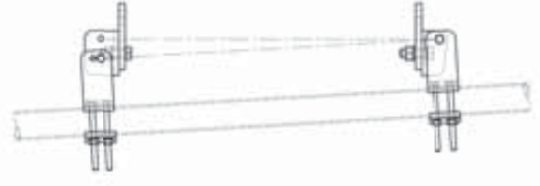
TAPERED 2' IN 20' SLOPE
