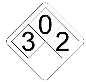
ALERTING SIGN (FOR CELL SITE BATTERIES)
