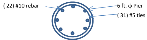
Monopole Pier Foundation
