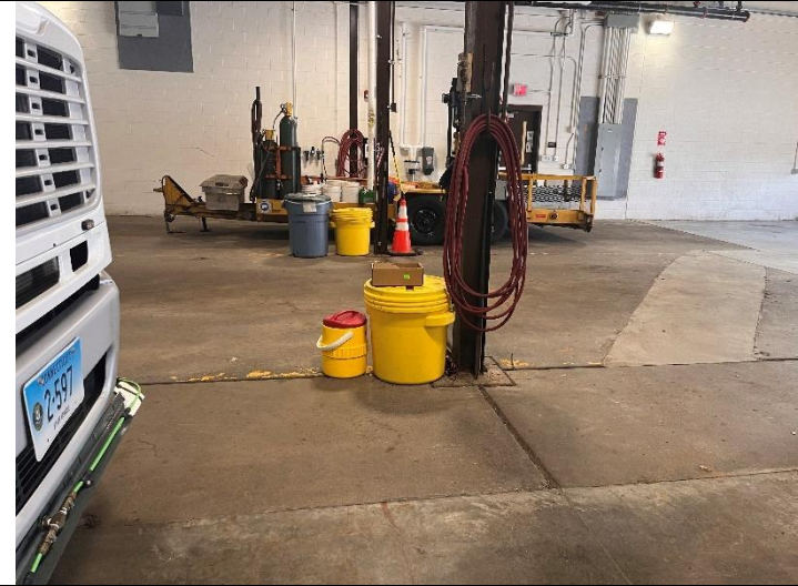
Keep spill kits available near vehicle maintenance areas/vehicle storage areas.
