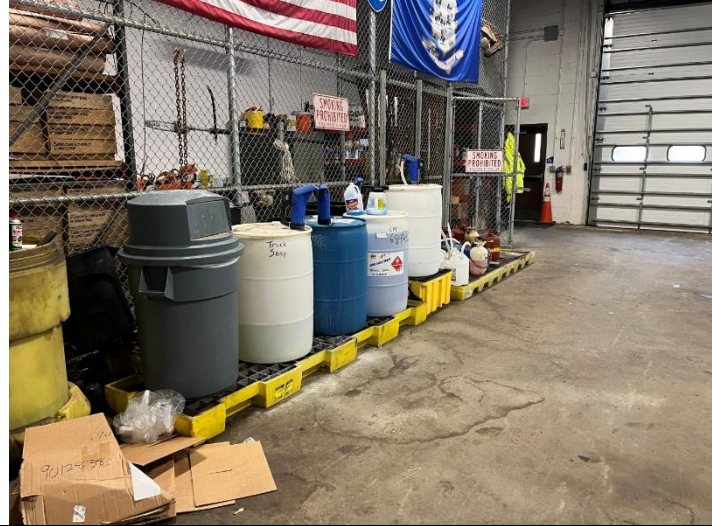
Store new and used petroleum products on impervious surfaces with secondary containment. Drain all parts of fluid into proper containers prior to disposal.
