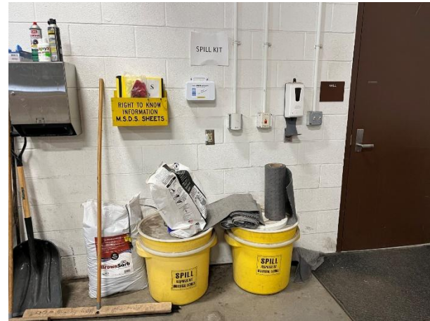
A complete spill kit should be stored inside the garage with a spark free shovel, Speedi-dri, absorbent pads, broom, and a disposal container.
