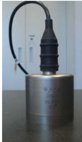
Figure 7: Piezoelectric accelerometer sensors
