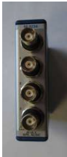
Figure 21: NI 9234 module for collection of piezoelectric accelerometers/strain gages data
