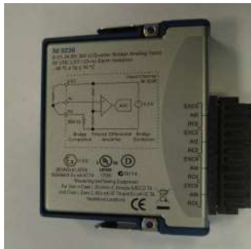
Figure 20: NI 9236 module for collection of foil Strain gages data
