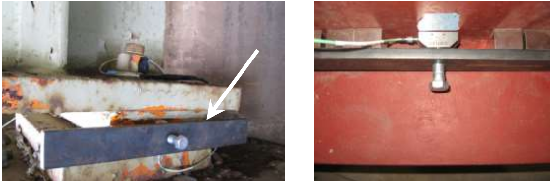
Figure 28: Magnetic mount to install piezoelectric strain sensors
