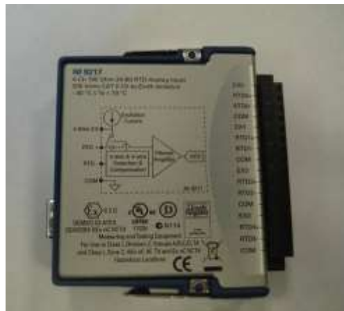
Figure 23: NI 9217 for collection of temperature sensors data
