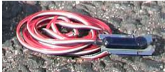
Figure 3: Foil strain gages used on the Meriden Bridge
