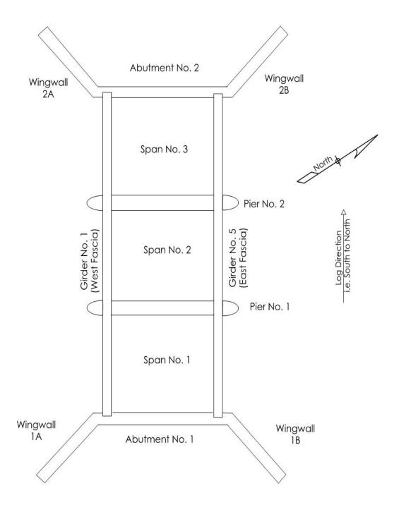
Figure 6.0a – Bridge Component Labeling System
