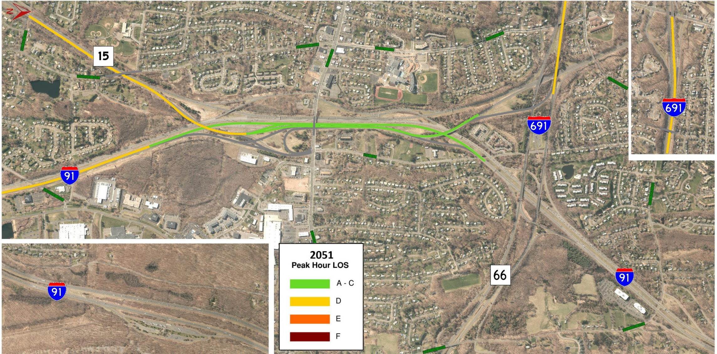
Critical LOS for AM or PM peaks selected for each highway segment, for design year 2051.
