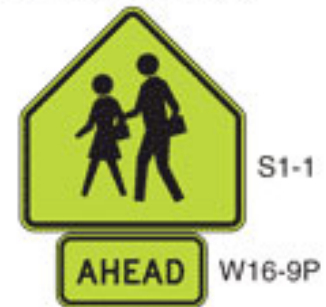
Figure 28: MUTCD S1-1 Sign and W16-9P Sub-Plate
