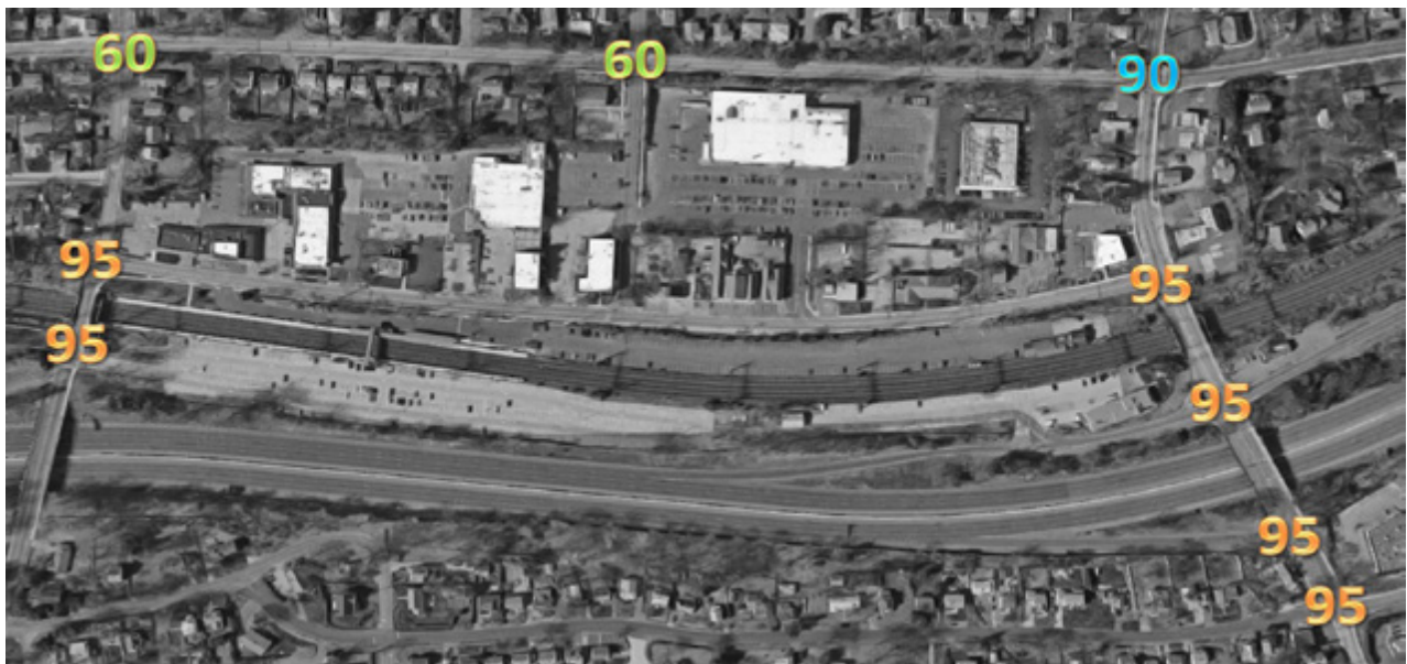
Figure 16: Existing Traffic Signal Cycle Lengths
