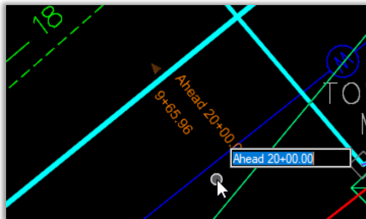
Figure 45 – Start Station applied to alignment
