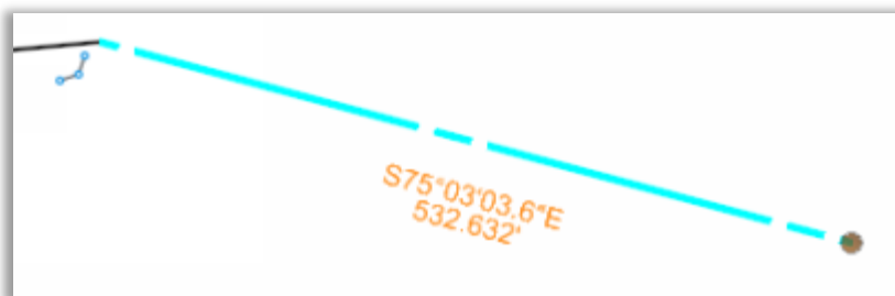
Figure 165 – Second line maintains its relationship if first is modified
