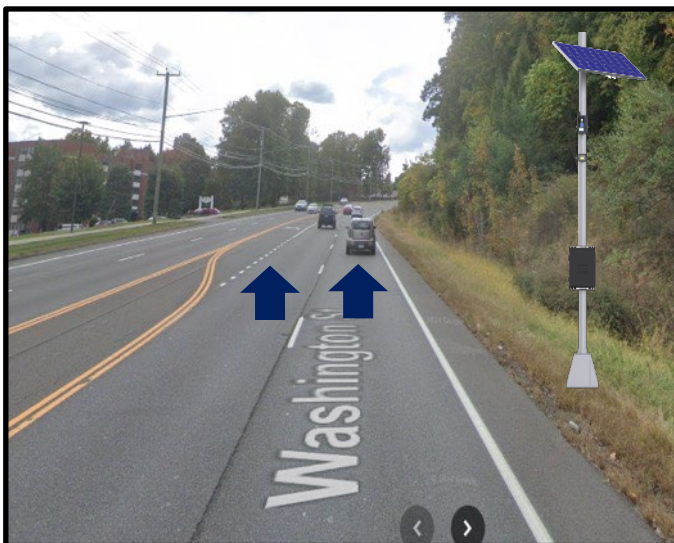
* Sample VR image of camera placement. Arrows indicate image capture for violating vehicle's direction of travel.
