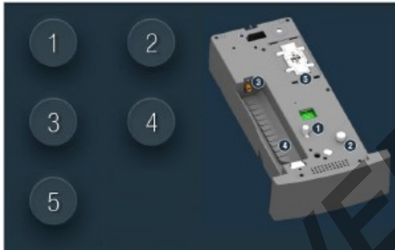
Figure 23. Steps for replacement and the location on the primary cartridge
