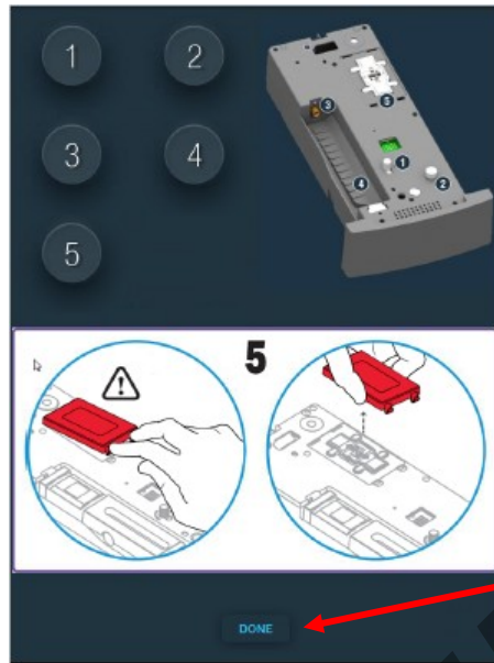
Figure 31. Selecting Done after removing the capillary cover
