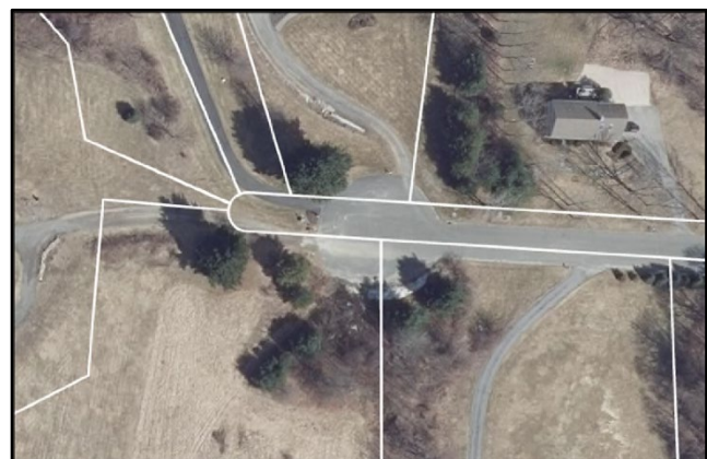
Misaligned parcel boundary with respect to the road ROW
