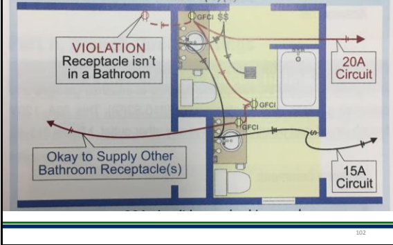
20A Bathroom Receptacle Circuit, Dwelling 210.11(C)(3)
