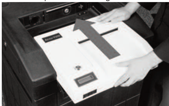
Step 8 – Slide the Optical Scan halfway into the ballot box
