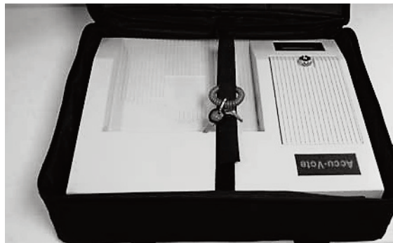
Step 18 – Place the tabulator back into its carrying case
