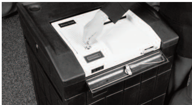
Step 16 – Replace and lock the printer cover
