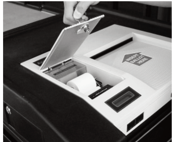
Step 12 – Unlock and remove printer cover.
