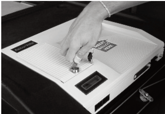
Step 12 – Unlock and remove printer cover.
