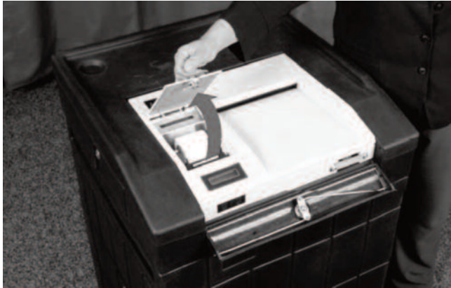
Step 8 – Unlock and remove printer cover
