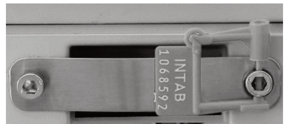
Step 5 – Check the tabulator memory card seal. It must match the number in the Moderator's Return
