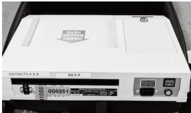
Step 4 – Unpack Optical Scan unit and inspect it. Check the precinct label, the seals, and the tabulator serial number. They must match the numbers in the Moderator's Return
