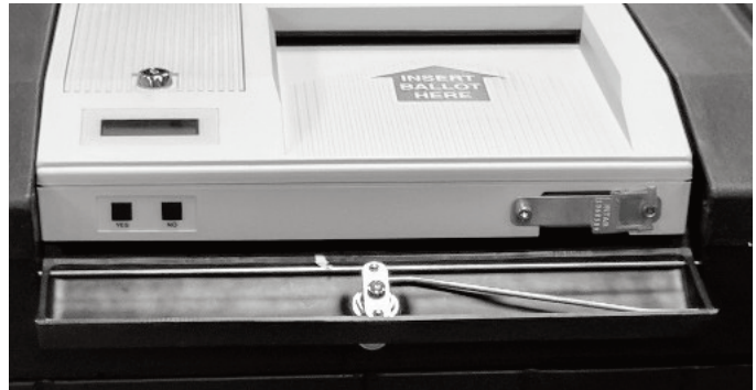
Step 19 – Slide the Optical Scan unit all the way back until securely seated
