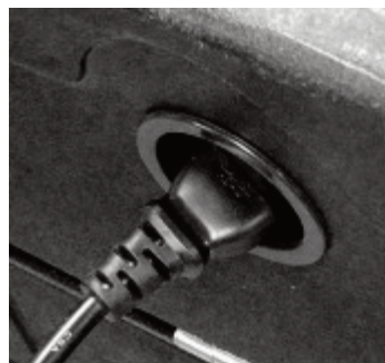
Step 9 – Feed the power cord through the tunnel in the back of the ballot box
