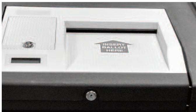
Step 20 – Close and lock retaining door
