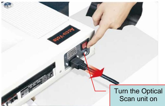
Turn the Optical Scan unit on
