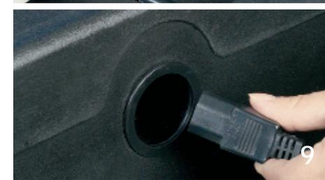
9 Turn off the AccuVote unit by pressing the red ON/OFF switch on the back of the unit. Unplug the power cord from the UPS unit, unplug the unit and remove the power cord. Repack the unit in its case.
