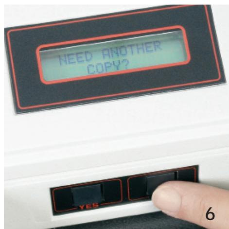
6 The final Summary Results Report will print automatically. When the tape is finished printing, the LCD on the AccuVote will display: "Need Another Copy?" Following directions from your local Elections Office push YES or NO on the unit.
