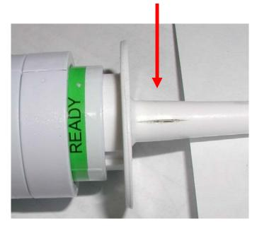
**Example of a Crack at the Base of the Syringe Tip**
