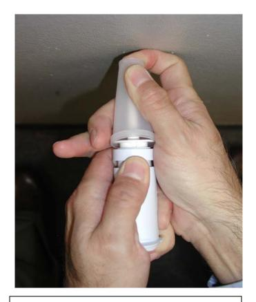
Step 3: Apply downward force with your thumb to create an opening 2/8 to 3/8" to view base of syringe tip and inspect for crack. Adjust angle to give best view of syringe tip.
