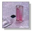
**Colorimetric tests** use a reagent which changes color depending on the concentration of the chemical being tested. The color is then compared to a standard to determine the concentration. Disinfectant and pH are usually tested using this method.
