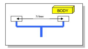
• <u>Secondary layer</u> of protection is required if the pool has a single blockable drain or has multiple drains less than 3 feet apart. Secondary layers of protection include:
