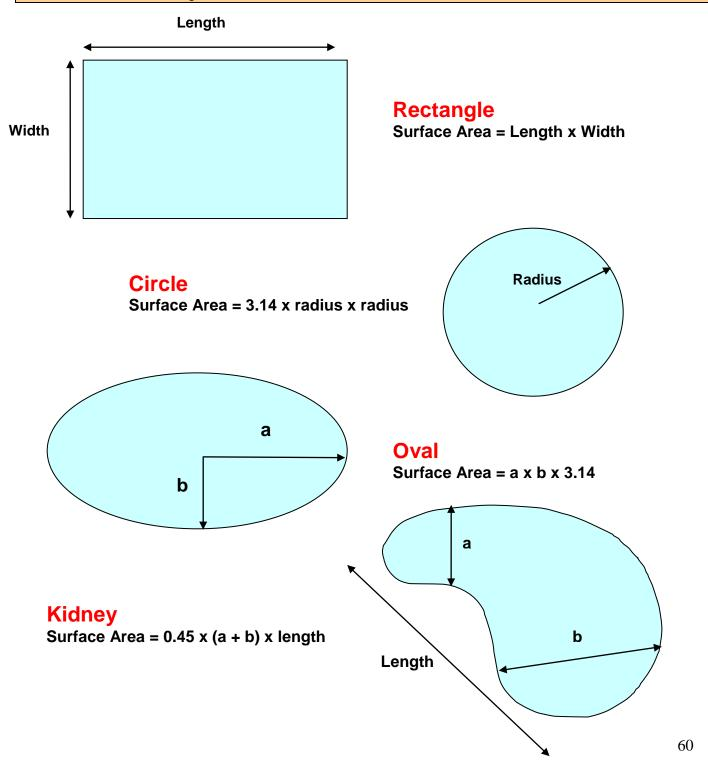
Some pools are a combination of common shapes requiring adding the sum of the shapes together to get the total surface area.
