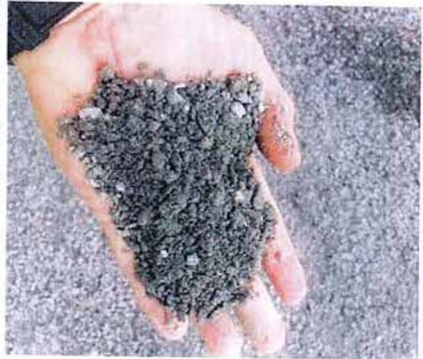
Typical field base top material after rain event
