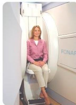
Figure 6. Resistive passively-shielded 0.6 T open magnet (Fonar Corp.)
