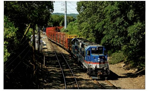
ABOVE: ConnDOT Brookville BL20GH 126 passes the searchlights that protect the east and west legs of the Devon Wye on the afternoon of March 16, 2015. These signals were taken out of service and removed when the Waterbury Branch received new signal upgrades and PTC.
