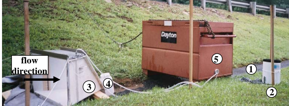
Figure 1. Sample collection apparatus. Apparatus was deployed in an asphalt stormwater conveyance gutter (1) to await initiation after 60 mm/h precipitation intensity detected by a tipping bucket rain gauge (2). Stormwater flow was measured with an H-flume equipped with a bubble flow meter (3). Flow exiting the flume via a dump cup (4) was sampled using a 12-position automated sampler contained within a secure box (5).
