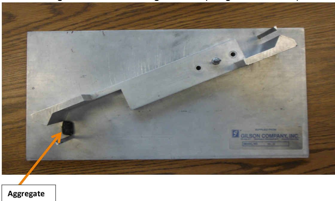
Figure 1. Flat and Elongated Test (Longest Dimension)
