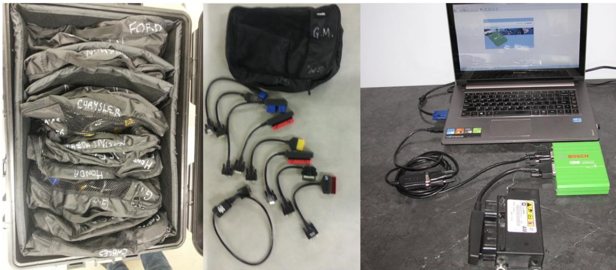
Figure 2: EDR Cables by Make and Model
