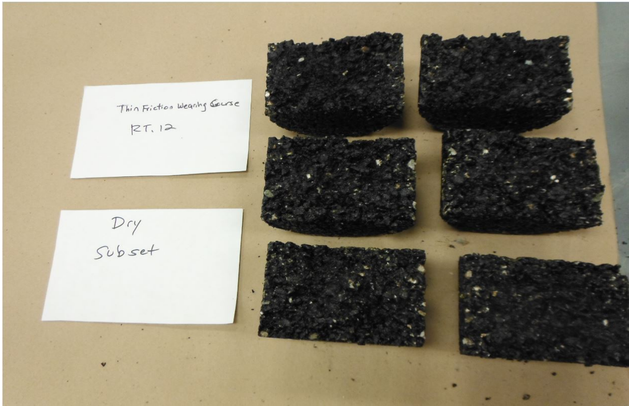
Figure 12. Unconditioned HFTL TSR Subset after Testing
