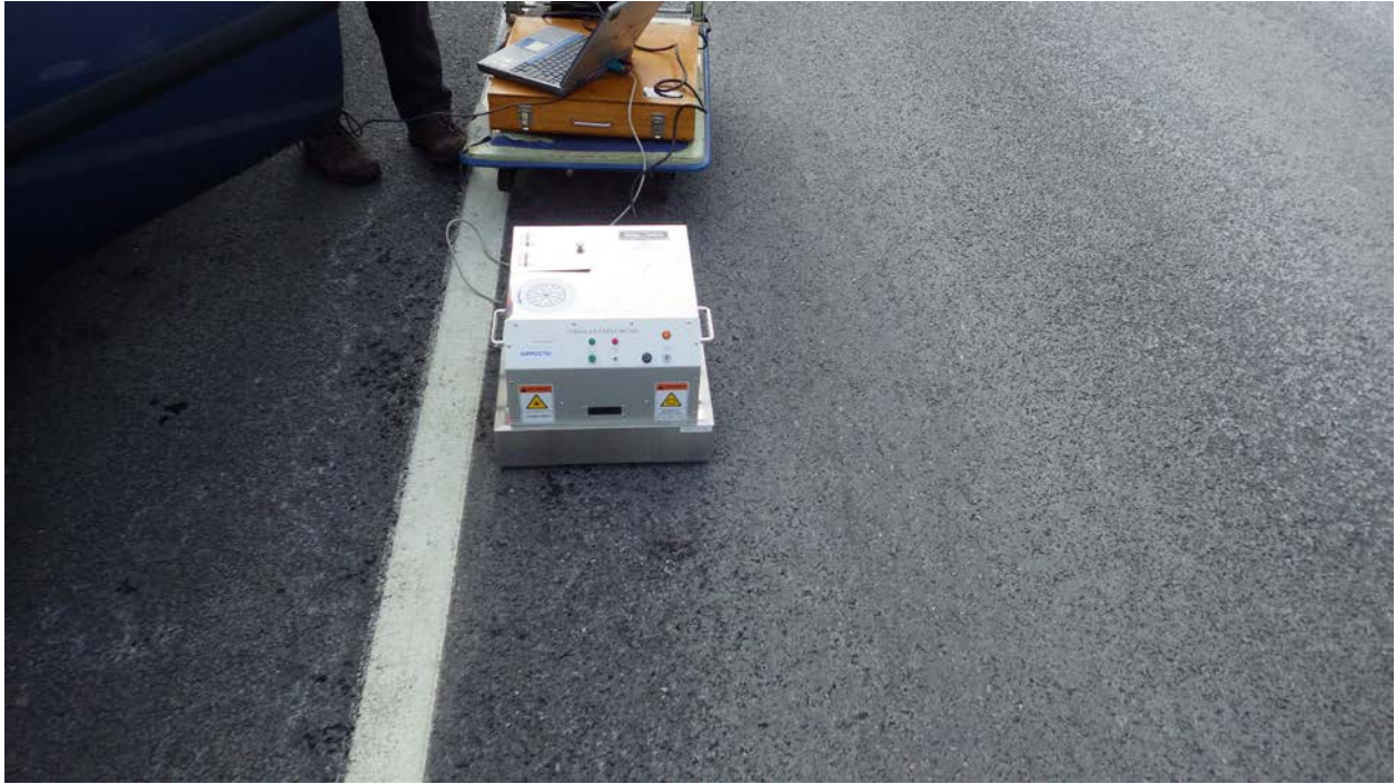
Figure 19. Circular Track Meter (CT Meter)
