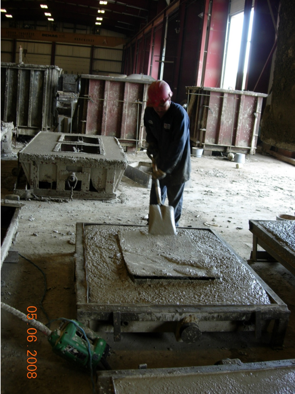
FIGURE 6 - Slight remixing and manipulation of SCC with a shovel for catch basin top.
