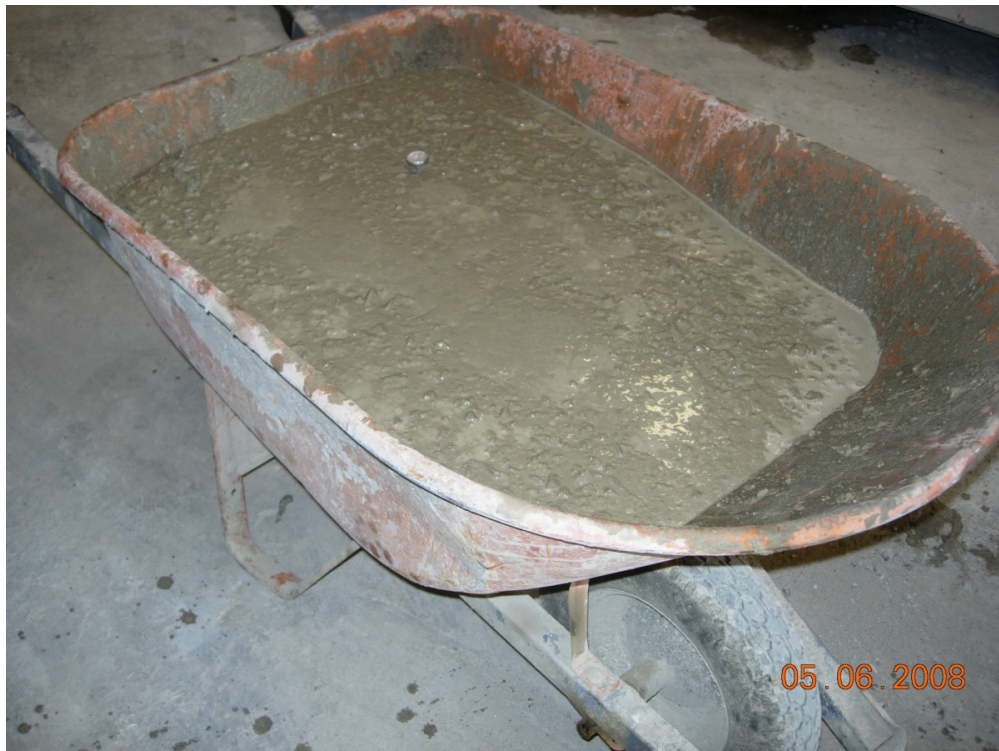
FIGURE 1 - Fresh sample of concrete in wheelbarrow and concrete temperature being measured with probe. Note: visible evidence of bleeding.
