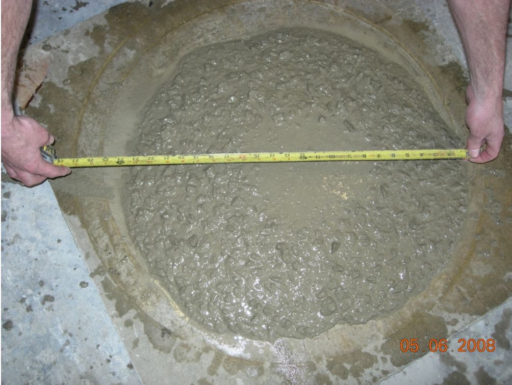
FIGURE 4 - Spread being measured from ASTM C1611. Slight bleeding observed as a sheen on the concrete mass, and segregation is evident in center of mass. VSI value between 1 (stable) and 2 (unstable).
