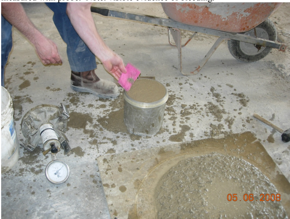
FIGURE 2 - Measuring bowl for determining air content by the Pressure Method filled, struck off, and prepared to have cover assembly attached.
