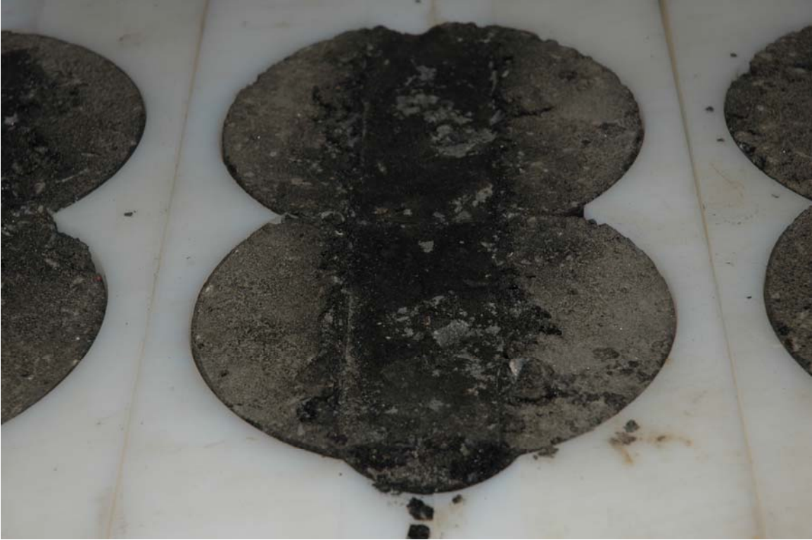
Figure 8. Hamburg Wheel Track Specimen after Testing
