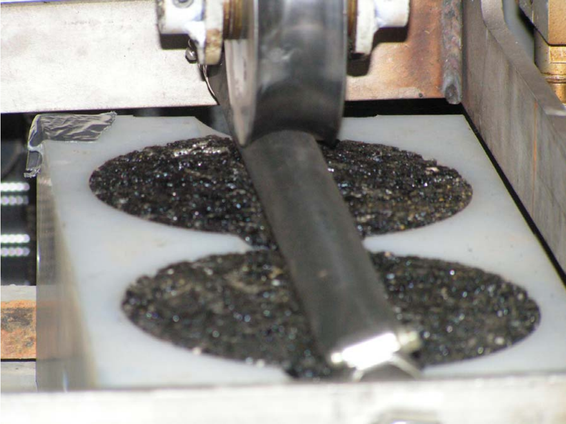
Figure 4. AASHTO TP 63 Close-up Pressurized Tube Over Test Specimen
