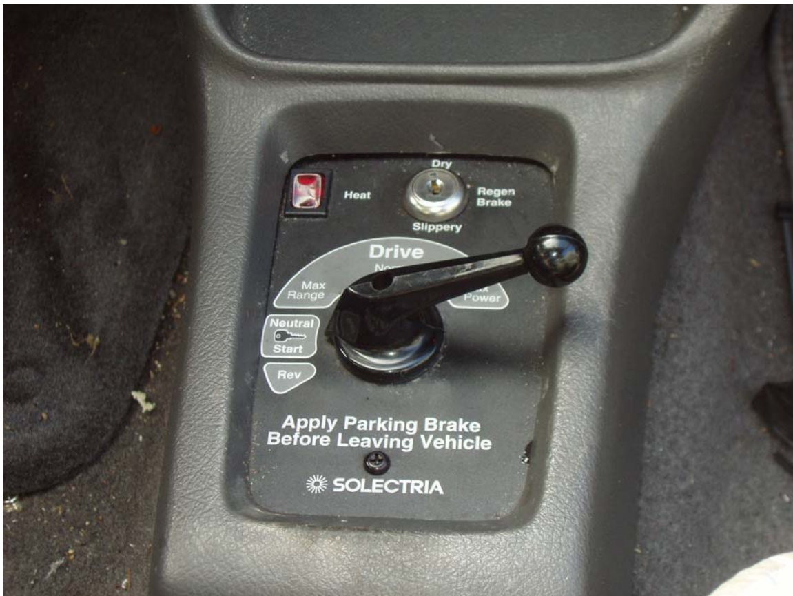
Figure 10 Photo of drive controller used in EV-3 and EV-5. Note the three modes: Max Range, Normal Range and Max Power.
