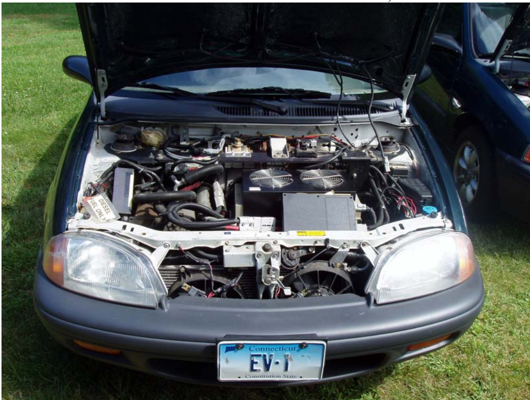
FIGURE C-2 Under the hood of one of the Phase 2 electric vehicles, EV-1.
