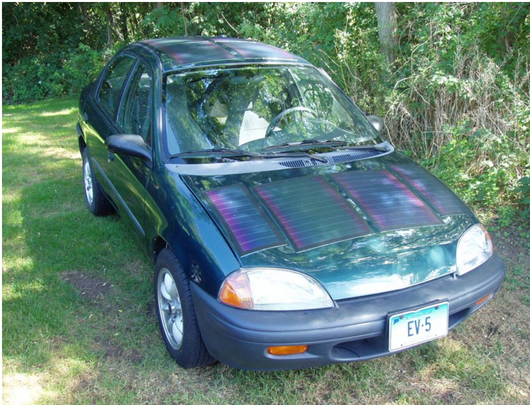
Figure 5 Photovoltaic laminates on Phase 2 battery-electric vehicle (typical of others).
