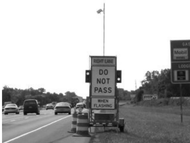
Figure 17: I-94 Dynamic Lane Merge Sign Photo courtesy of FHWA (Federal Highway Administration)
