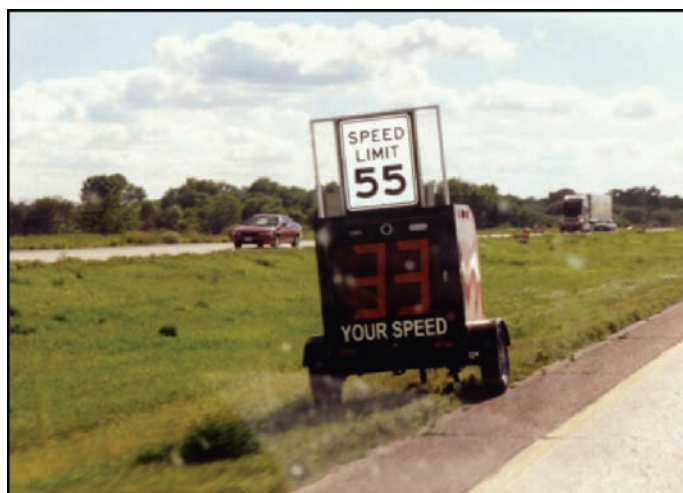
Figure 2: SpeedGuard Radar Speed Reporting System From the report “SpeedGuard Radar Speed Reporting System - Nebraska” (McCoy, P.), with permission from Geza Pesti, Texas Transportation Institute
