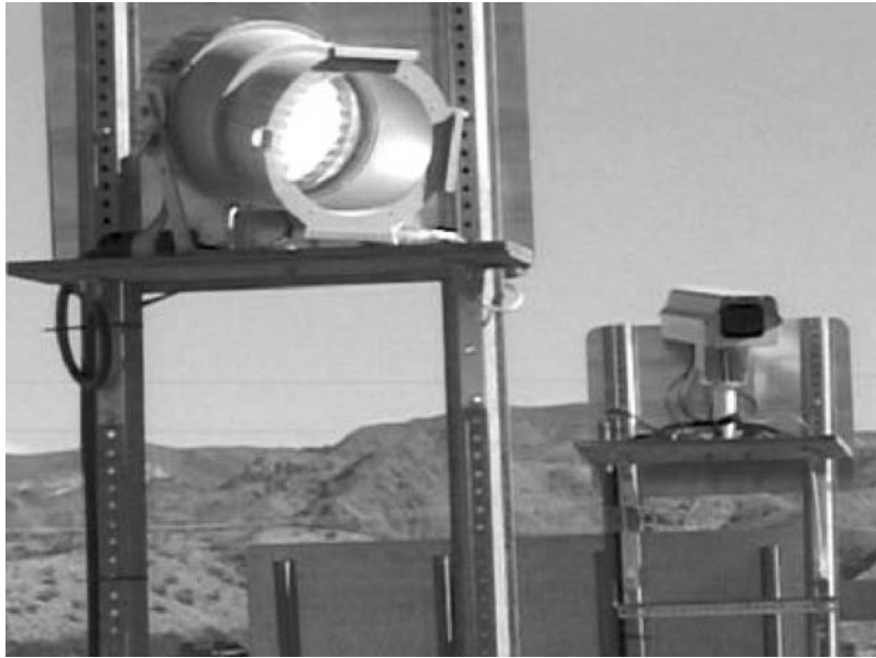
Figure 16: Light and Camera Used to Collect License Plate Data Photo courtesy of FHWA (Federal Highway Administration)
