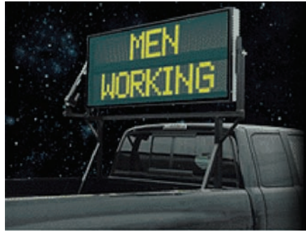
Figure 18: An Example of a Vehicle-Mounted PVMS ( http://www.ver-mac.com/en/products/tcms.html )
