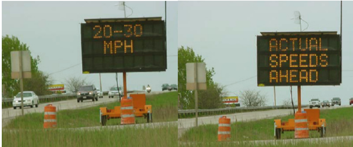
Figure 6: Variable Message Sign (VMS) Messages from Intellizone
