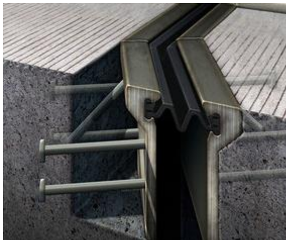
Figure 6: Typical strip seal joint (DSB 2015)
