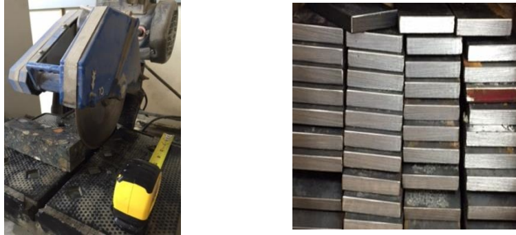
Figure 12: Fabrication of coupons for experimental testing
