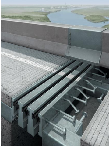
Figure 8: Typical modular bridge joint (DSB 2015)
