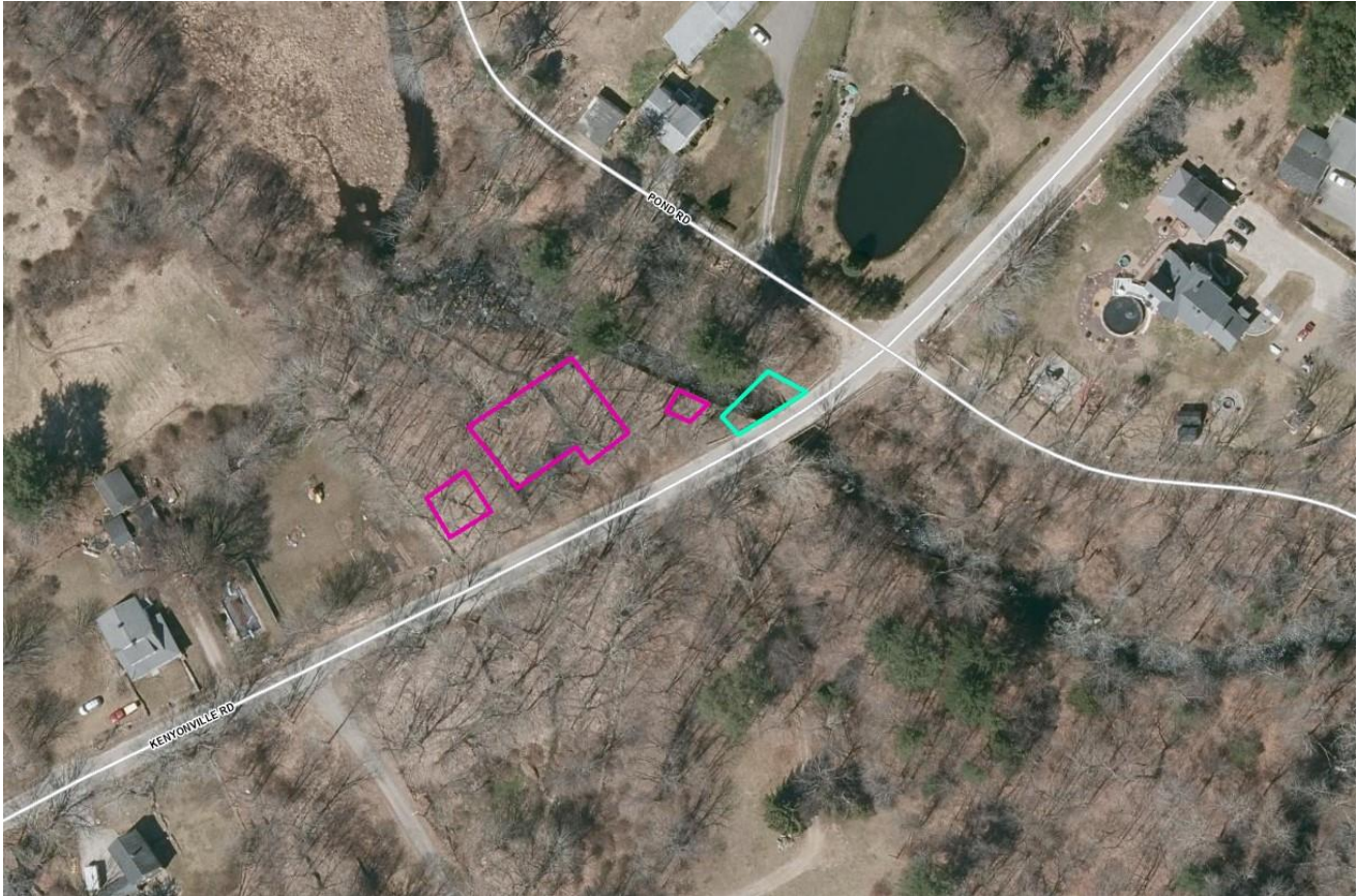
Figure 7: Aerial photograph showing locations of mill features to be avoided (red) and area of stone retaining wall to be removed and reconstructed (green).
