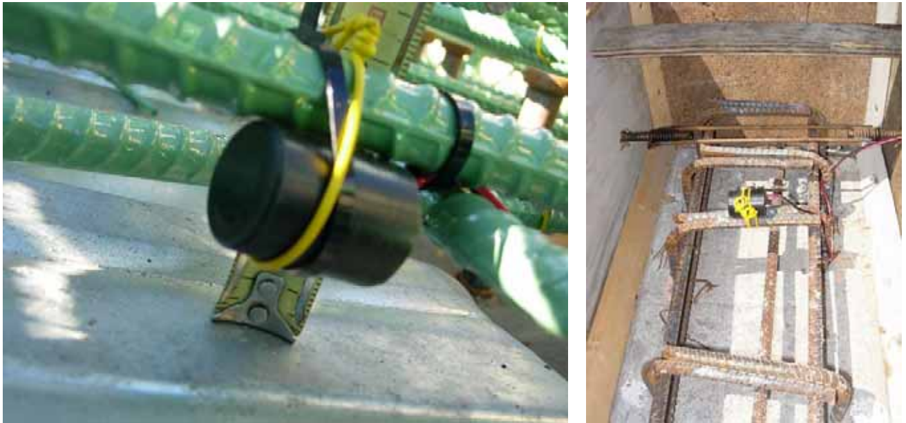
Figure 7 MAT-02-1H28D Loggers attached to reinforcing steel.
