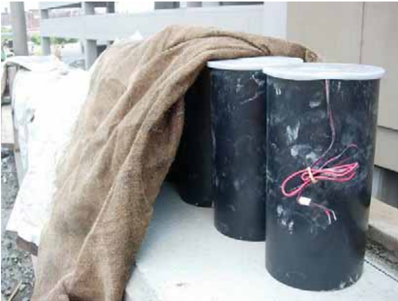
Figure 45 Companion specimen with probe installed cured alongside acceptance specimens.
