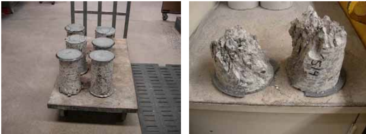
Figure 37 Drilled cores after compression tests.
