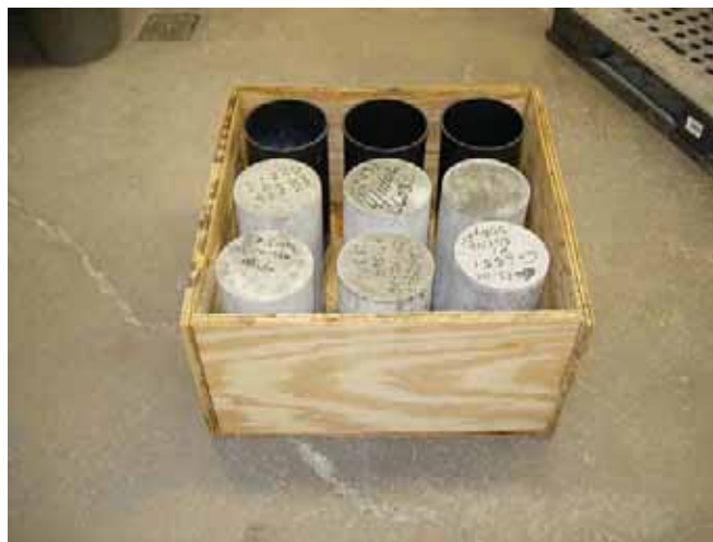
Figure C-1 Photo of curing box with 9-specimens inside.
