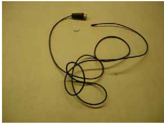
Figure 22 IQ32TE, tag (left) and probe (right).
