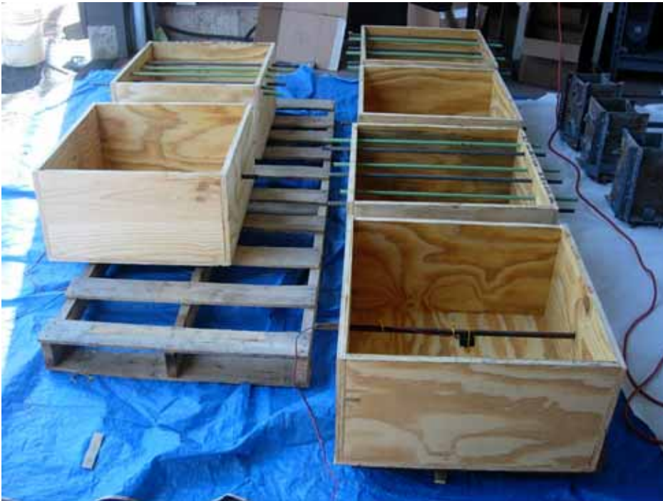
Figure 32 Forms for concrete blocks.
