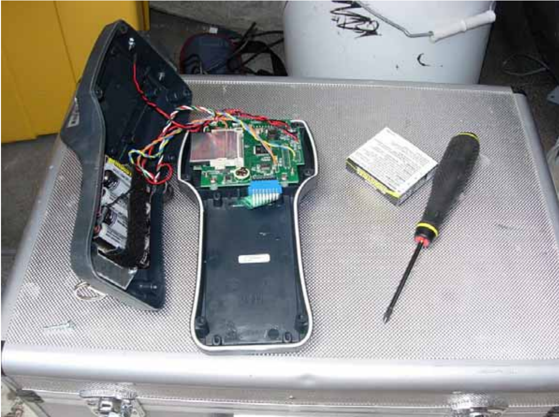
Figure 6 KIT-02 Reader opened to change batteries.
