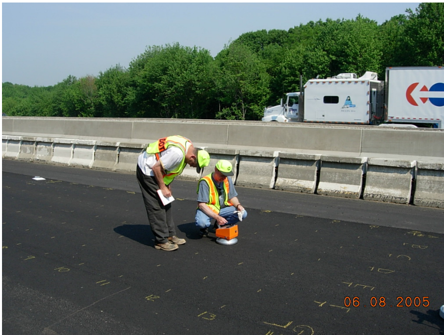
Photo #8, Density Measurements with PQI, I-84
