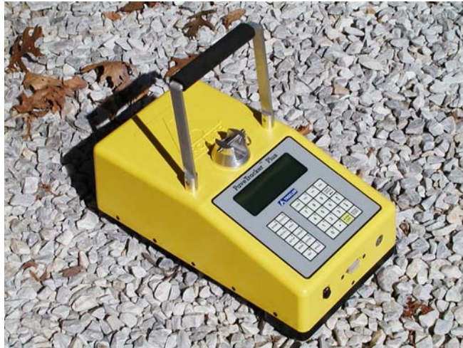
Photo #3, ConnDOT PaveTracker Plus, Model 1701B
