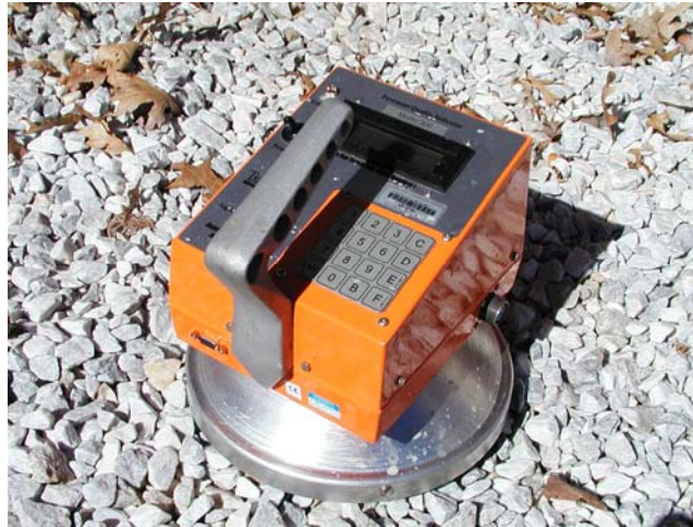
Photo #4, ConnDOT Pavement Quality Indicator (PQI), Model 301+
