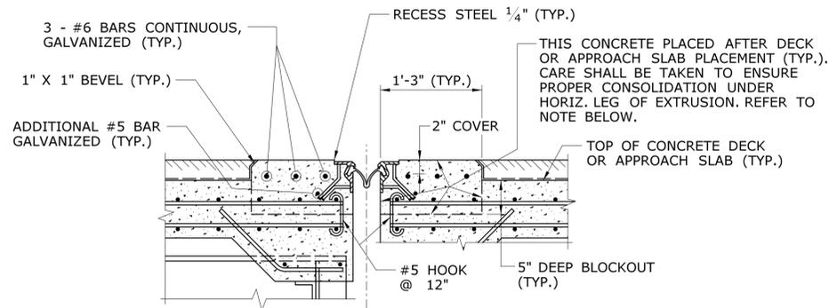
**SECTION - STRIP SEAL IN CONCRETE HEADER**
