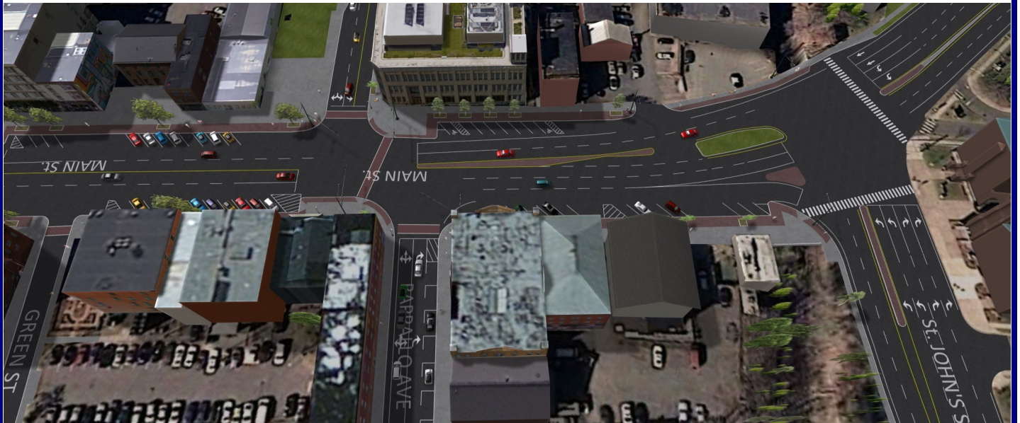
FIGURE 8—SAINT JOHN'S SQUARE GEOMETRIC REALIGNMENT AND ADDITIONAL TURN LANES
