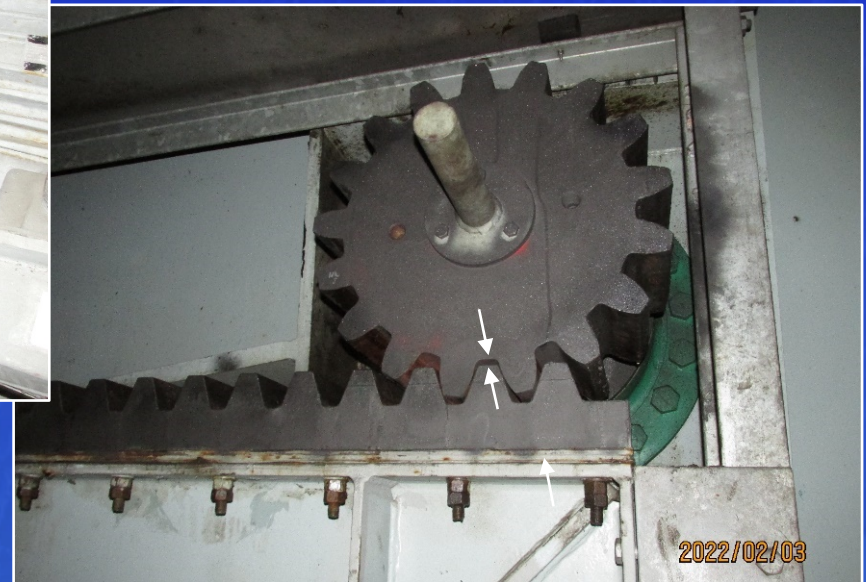
Reduced Rack and Pinion Tooth Root to Tip Clearance. Remove Rack Shims
