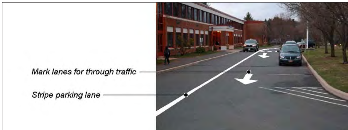
Figure 2: Stripe parking lane at school entrance. Reserve center of driveway for through traffic. Monitor parents during drop-off and enforce full use of parking lane for drop-off.
