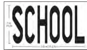
School zone speed limit signage and pavement markings would increase driver awareness and slow speeds approaching crosswalks.
