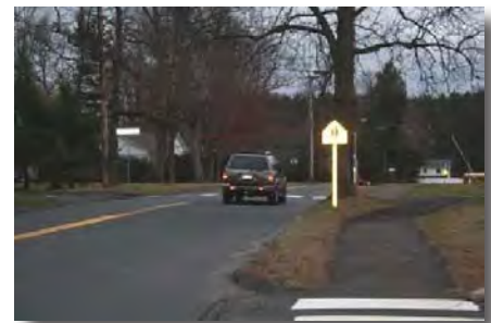
Crosswalk signage, while present, was not located directly at crosswalk locations.
