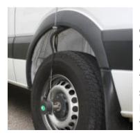
The Distance Measuring Instrument (DMI) measures ARAN chainage or linear distance travelled. It is the most basic and yet one of the most important measurements made by every ARAN vehicle. The DMI allows a vehicle to move at variable speeds in traffic and collect data safely without data corruption due to speed changes. All data must be accurately referenced to its location on the road and the DMI is an integral tool in carrying out that task.
