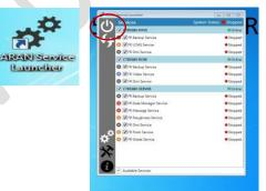
i. Run ARAN 9000 system **Diagnostics** and check for any warnings or errors. *Allow* **15** *min. idle time for GPS accuracy and computer communications*.
