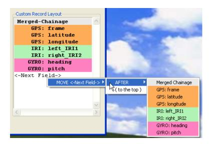
The individual **Geometric Data Fields** can similarly be moved to any position in the Custom Record Layout box, but what makes them unique is that they can be removed from the box (minimum of one field for each Data Stream will still apply). Aside from pushing the **Clear** button which removes everything from the box, these can be removed by clicking on the one you wish to remove and then simply clicking the **Delete** option in the menu that pops up, as pictured below.
