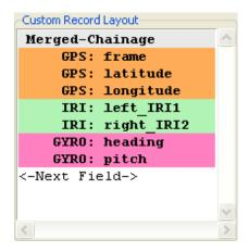
The **Merged-Chainage** field at the top of the box is unique in two ways. The first is that unlike the individual colored bands of geometric data, the Merged-Chainage field is actually comprised of the chainage numbers accompanying each of the Data Streams represented (except for the Van information Data Stream). Below: the picture on the left shows the menu that appears when you click the **Merged-Chainage** Line and pictured right is the expanded Merged-Chainage field.
