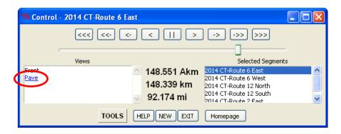
As mentioned earlier in this manual, clicking **Pave** will open up a new window displaying images of the pavement taken at approximately the same point along the route as the front image currently on display.
