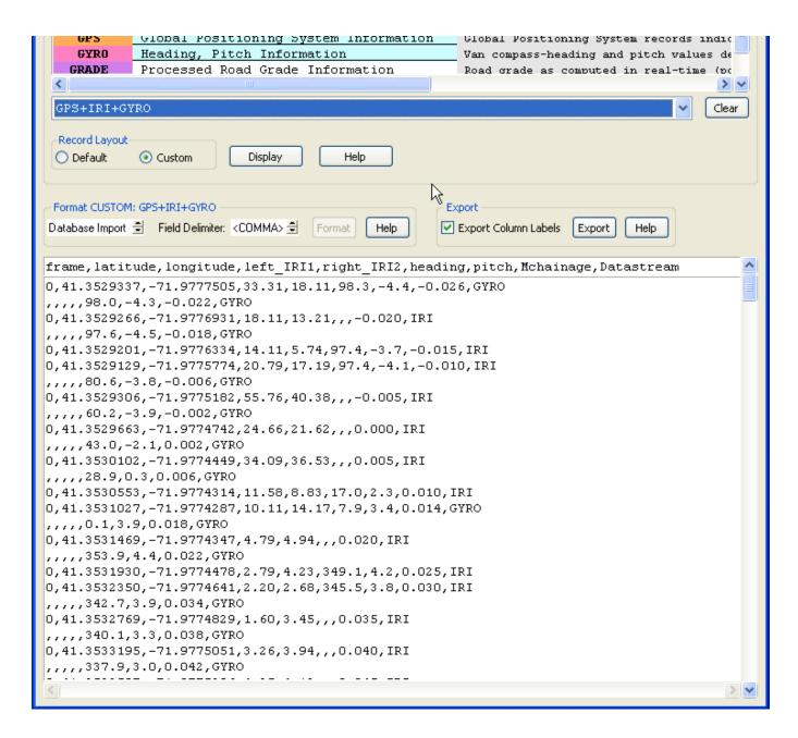
After you've formatted the data to your liking, check or uncheck the **Export Column Labels box** and then press the **Export button**. Unchecking this box simply removes the headers from the exported document.
