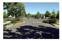
*Pros* :: Narrowed lanes can slow vehicle speeds; Breaks up driver sight lines; Increases pedestrian and motorist visibility.
