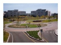
roundabout and the geometry is specifically designed to restrict speeds. Modern roundabouts may be used in place of traffic signals at higher volume roads.
