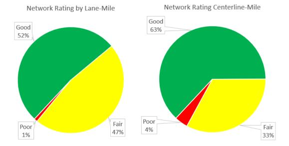
Figure 2-6 Conditions of CTDOT-Maintained Roadways (2019) Using the PCI, by Lane Mile and Centerline Miles (Excludes Town Roads)
