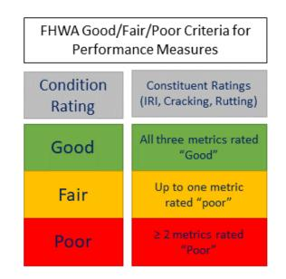
Figure 2-9 FHWA Performance Measure Criteria for Good/Fair/Poor Ratings
