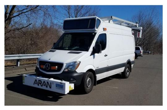
Figure 1-2 CTDOT Photolog Vehicle (One of Two Vehicles Currently Utilized)
