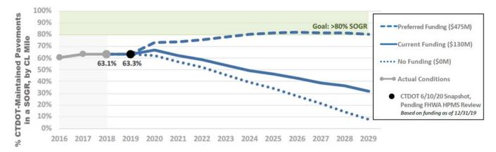
Figure 3-1 Connecticut Pavement Performance Projections for the CTDOT Maintained Network (from June, 2020 CTDOT Asset Fact Sheet)
